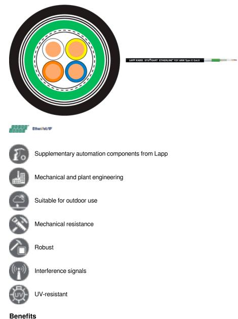
Can be used for Industrial Ethernet in harsh industrial environments EMC-optimised design With armouring for improved rodent protection Screened against interference 2pair: 10/100 Mbit/s for Industrial Ethernet
