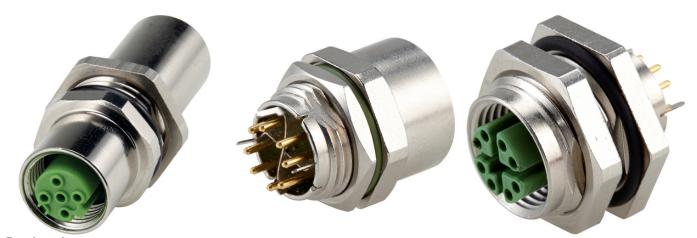
**Product features** Designs for front and rear wall-mounting M12 panel feed-throughs for direct connecting with PCB Can be used for Industrial Ethernet in harsh industrial environments Housing: zinc die-casting, grey
